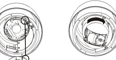
**IMPORTANT!** Power the dome (heater fans turn on) and check it performs its homing routine. During this routine, the camera lens moves up into the dome housing, down to the floor, pans slowly, and moves up to its home position. The controller can then be used to call up and control the dome.
